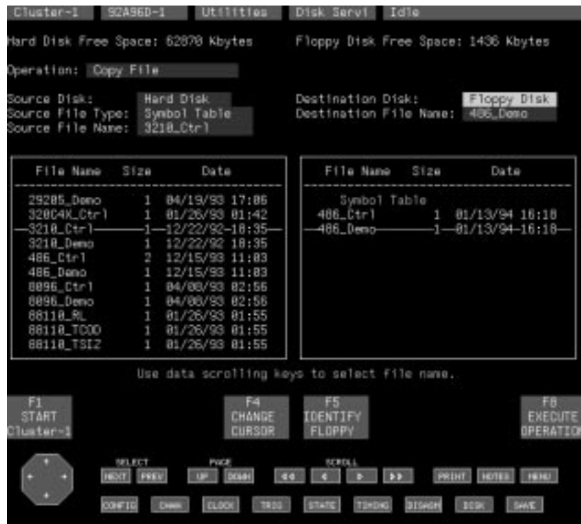
Figure 3–15: Disk Services Menu: Copy File Operation
